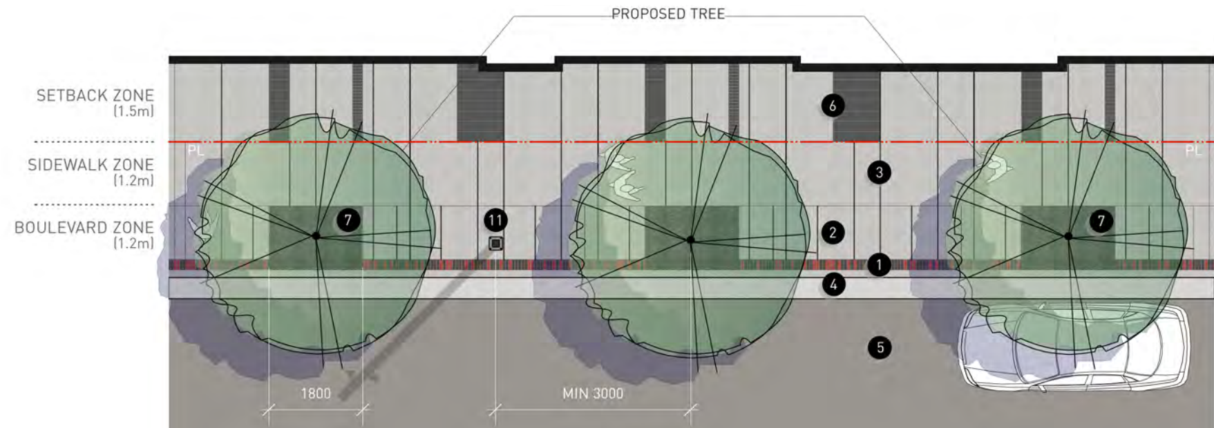
Plan: Typical Widened Sidewalk Replacement: North-South Streets | Scale 1:100
